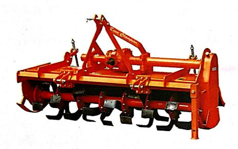
SHAKTIMAN ROTARY TILLER, MODEL: SRT-6(180)/SS CD SC SINGLE SPEED, CHAIN DRIVE, CENTRALLY MOUNTED
